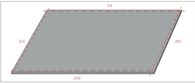
Image 11: Correct order to remove slabs sides
