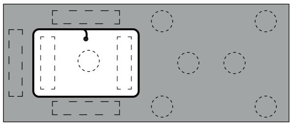
Image 16: Cut-outs with CNC. Suction cups placement
