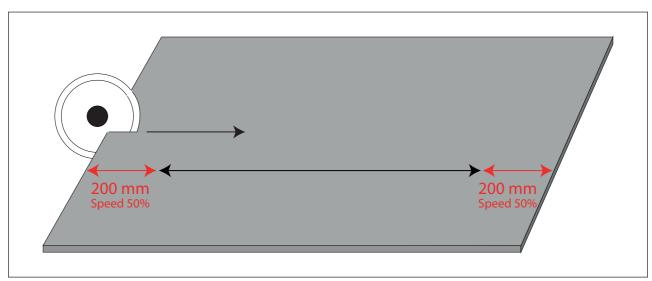
Image 12: Cutting speed recommendations for 12 mm
